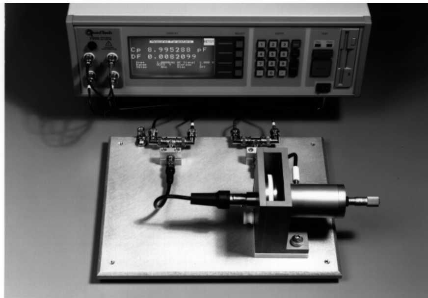
Figure1: IET Labs 7600 Precision LCR Meter connected to Dielectric Products LD-3 Cell
